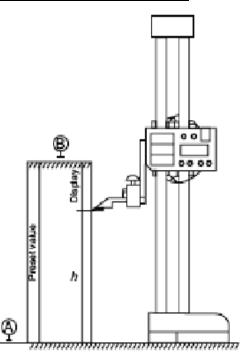
• Measuring procedure with preset value "b" Turn the hand wheel, let the bottom plane of the scriber contact with the base plane A, then do the following operations:
